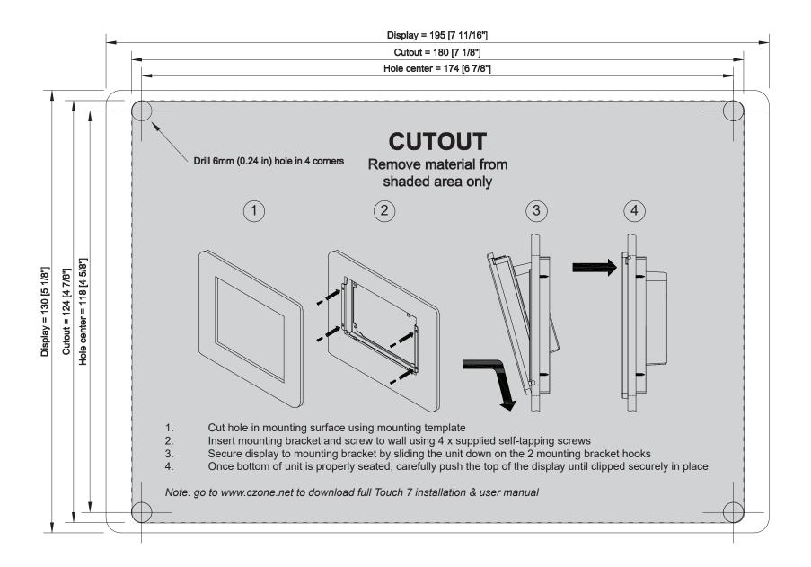
IMPORTANT! Ensure this printed mounting template is true to scale before cutting any mounting surface. Use a ruler to check the dimensions are correct
